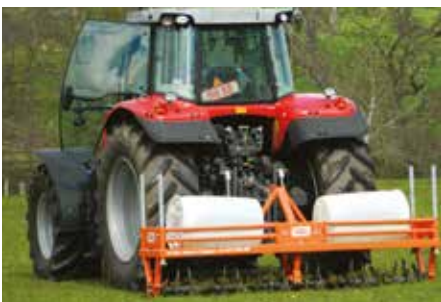
Figure 2.14. A soil aerator being used to aerate a field previously subject to heavy grazing pressure and compaction (© Tweed Forum).
